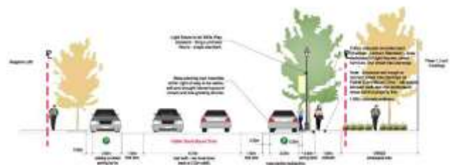
A cross section drawing for the CIGI Master Plan provides an effective technique to evaluate streetscape design and road function (including underground utilities).
